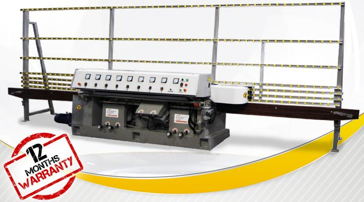
TThe Edge Pro 8 is a quality machine that will match any machine in the market. Designed for grinding and polishing bottom edge, fine grinding arris of flat glass.
